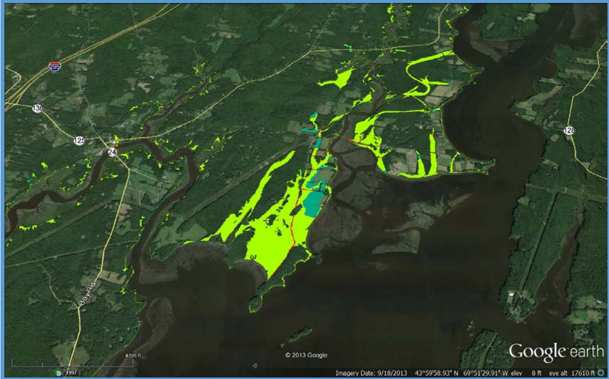
Figure 18: 2100 Predicted Inundation of Natural, Agricultural, and Developed Lands with 3.3 feet (1.0 m) of Sea Level Rise Alone, illustrating Table 6, rows 2 & 3. Total Water Level = 10.8 feet above MLLW.
