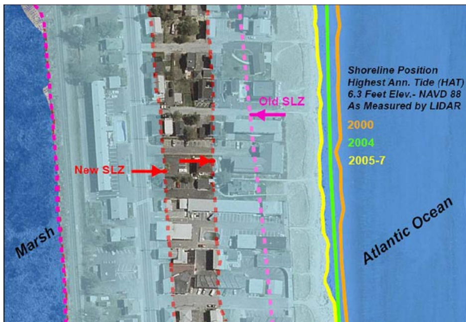
Figure 24: East Grand Avenue Area, Old Orchard Beach, Maine. Depiction of Old Shoreland Zone Boundary (purple), and New Shoreland Zone Boundary (red), Now Set 250 feet Horizontally Distant from the Level of the Highest Annual Tide. Highest Annual Tide was set at a contour height of 6.3 feet NAVD 88, using NOAA LiDAR data. From SMRPC.
