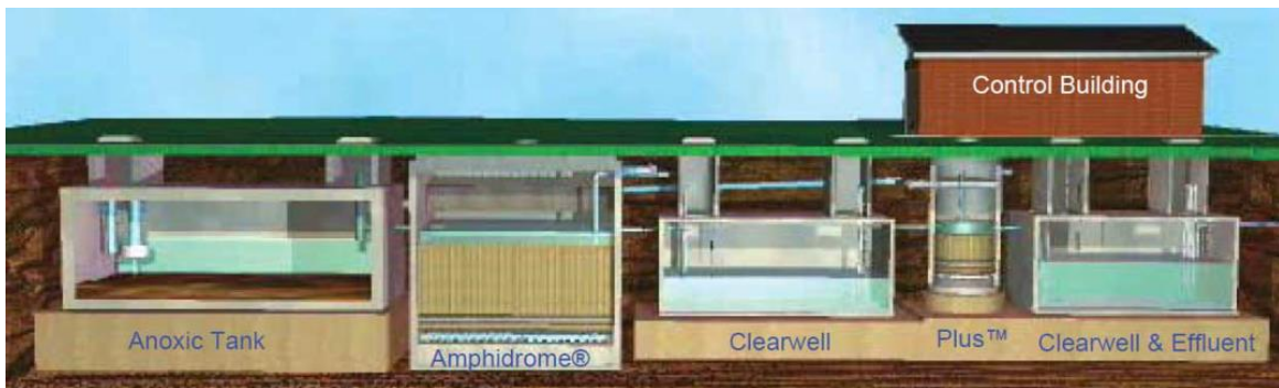
FIGURE 3-2 SECTION VIEW OF TYPICAL AMPHIDROME SYSTEM 1
