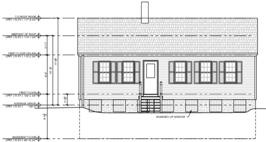
2 EXISTING SOUTH ELEVATION 10'-10"
